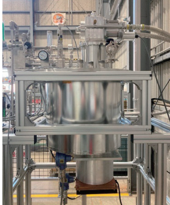
液化水素の蒸発ガス抑制装置の外観 Photograph of boil-off gas suppression unit for liquid hydrogen
