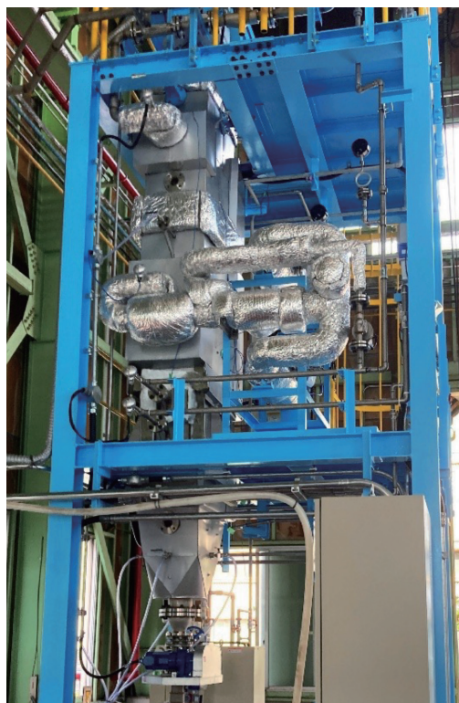
移動層化学蓄熱反応器ユニット Bench-scale reactor of moving-bed thermochemical energy storage
