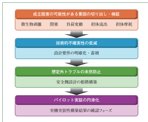
図6 実機実装を見据えた高負荷担体式嫌気処理の研究開発アプローチ Research and development approach for establishing the practical implementability of high-load carrier anaerobic treatment system
