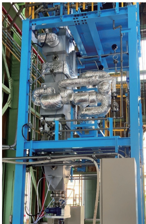
移動層化学蓄熱反応器ユニット Bench-scale reactor of moving-bed thermochemical energy storage
