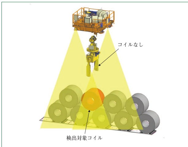
図2 コイル形状認識の機器配置 Equipment configuration for coil shape recognition
