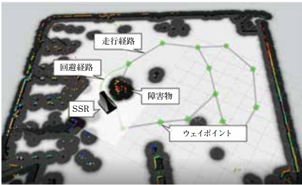
図2 SSRの自律移動 Autonomous moving of SSR
