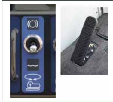
図4 旋回操作性を向上させる機能 Function for improving turning operability
