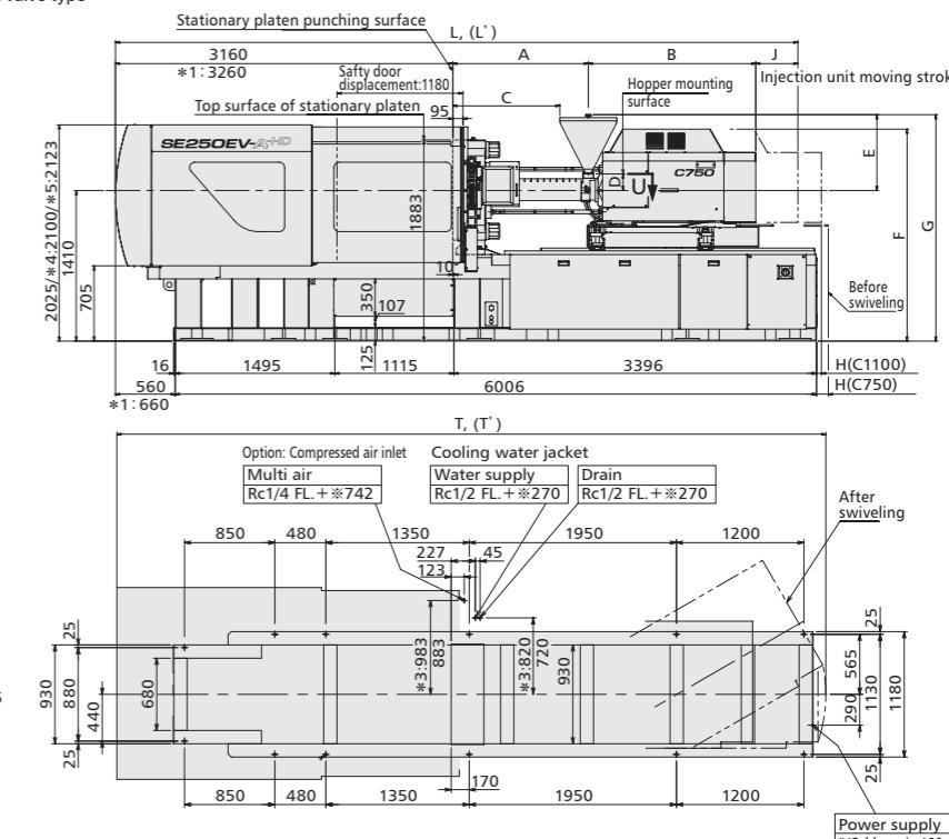
The figure marked with an asterisk (\*) shows the case of using no leveling pad.
