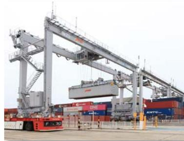
RTG = Rubber Tired Gantry crane
