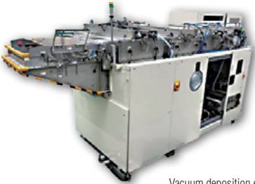
Vacuum deposition equipment for forming electron transport layers
