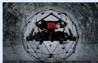
Inspection of the inside of furnaces by using a drone
