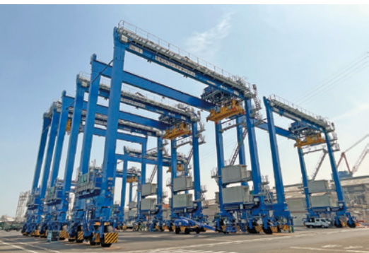
Remote-controlled Rubber Tired Gantry crane (RTG)
