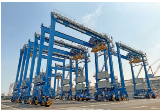
Remote-controlled Rubber Tired Gantry crane (RTG)
