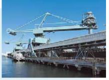
Continuous Ship Unloade (picture of the same type of unit already in operation
