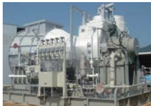
Steam turbine for power generation
