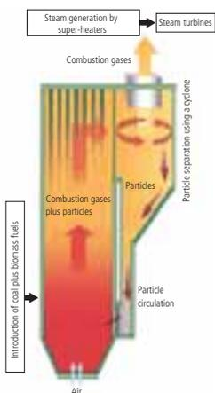
**CFB Boilers:** These boilers are compatible with low-grade coal (with high moisture content, low calorific value, etc.) and many other energy fuels that could not previously be burnt efficiently and stably in conventional boilers. The latest CFB boilers can handle even tires and other waste-based fuels as well as biomass-based fuels, both of which are being increasingly used in the place of fossil-based fuels. Accordingly, CFB boiler systems are gaining increasing recognition as
