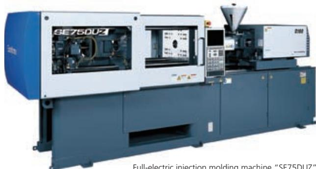
Full-electric injection molding machine "SE75DUZ"
