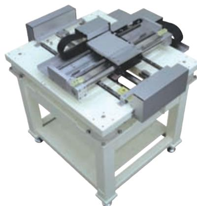
XY stage for inspection and repair system "TL Series"
