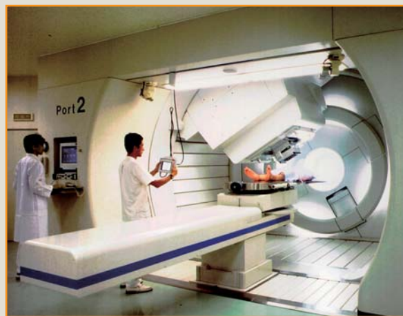
Irradiation system with rotating gantry (National Cancer Center Hospital East, Japan)
