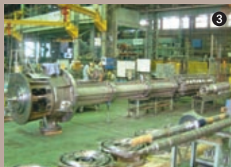
Vertically suspended multistage pump (Model: CZ)
