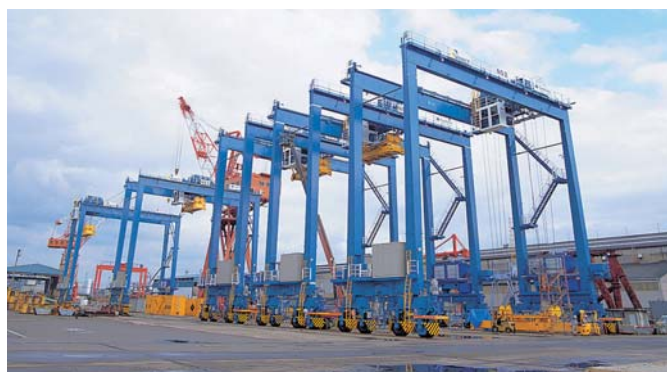
Rubber Tyred Gantry Crane (RTGC)
