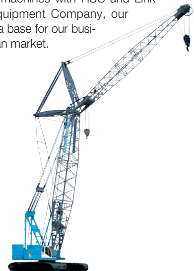
250ton-Type Crawler Crane
