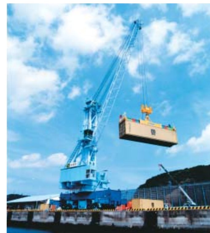
Tire mounted jib crane for Aburatsu Port (Miyazaki Pref.)
