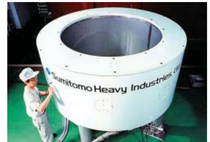
Superconducting magnet for silicon single crystal growth
