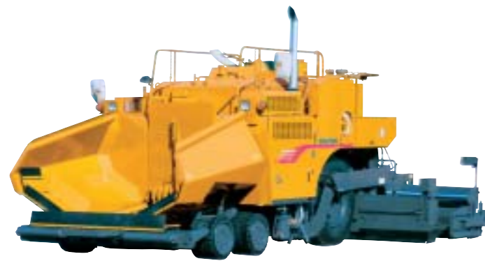
Road Paver with tack coat spreader
