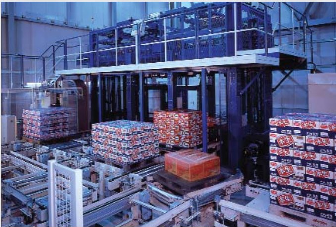
Automated picking system for liquor and beverage Cartons and plastic cases automatically picked and stacked
