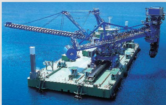
"KAIOSEI NO.2" - 3,000m 3 /h Continuous Bucket Elevator Reclaimer
