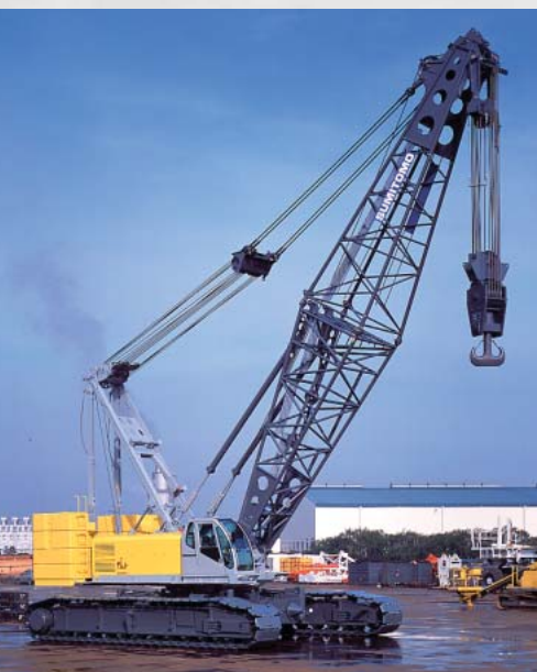
crawler crane SC2000-3
