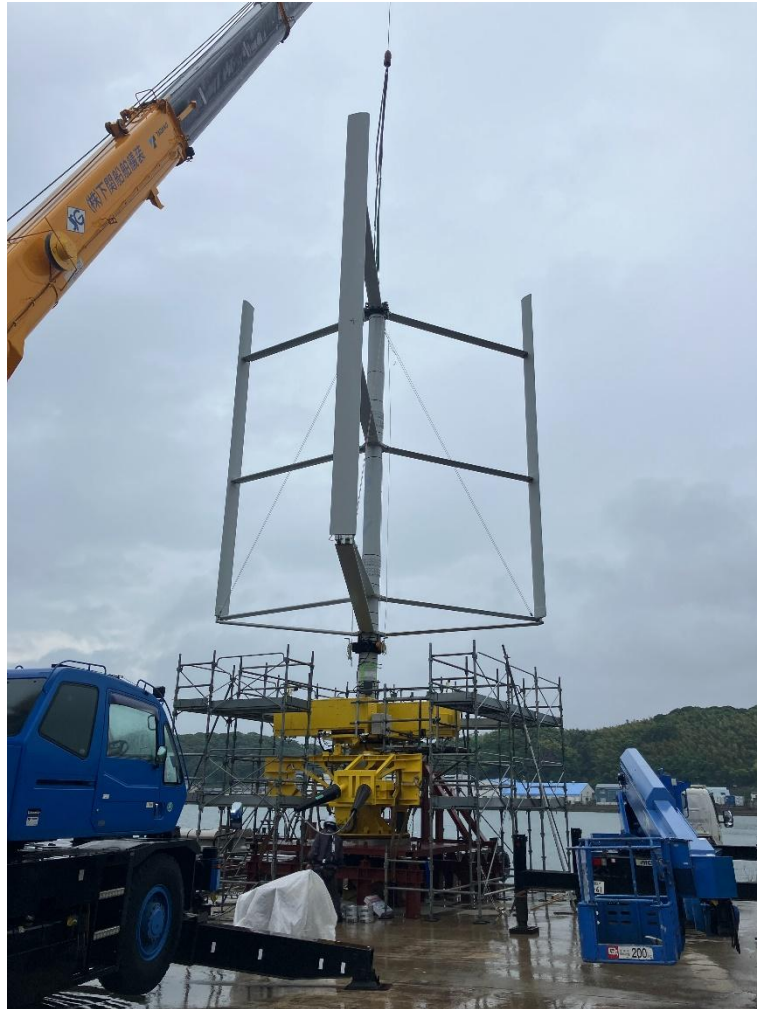
Onshore testing of the experimental FAWT
