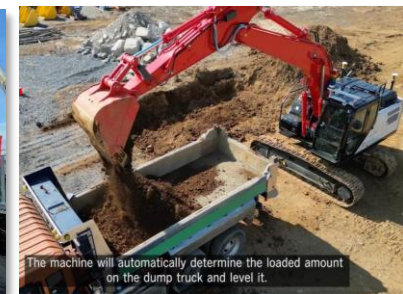
Remotely controlled, autonomous prototype hydraulic excavator
