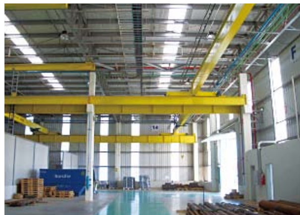
Speed reducer factory in Brazil With the skylights in the ceiling and walls, lighting inside the factory is unnecessary in daytime.
