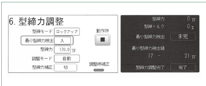
図3 最小型締力検出機能 Function for the detection of minimum clamping force
