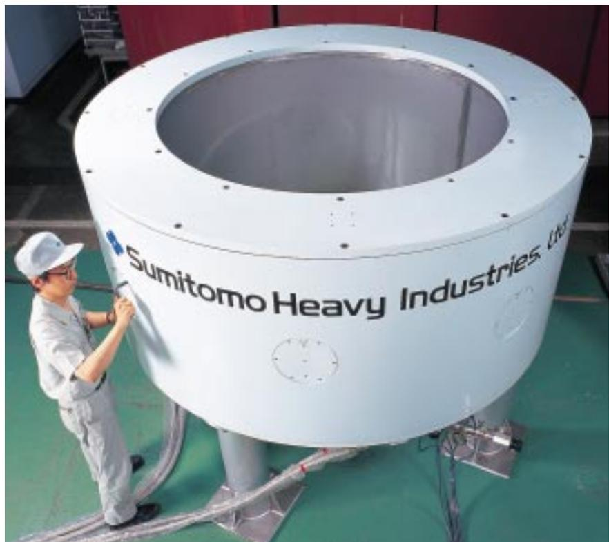
Cryocooled superconducting magnet
