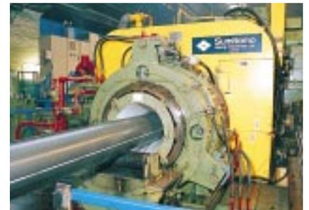
Milling cutter for 20" ERW mill for British Steel Tubes & Pipes
