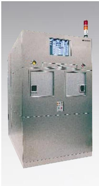
Cryogenic argon aerosol cleaning system
