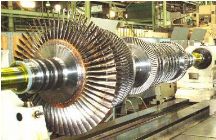
Steam turbine for power generation
