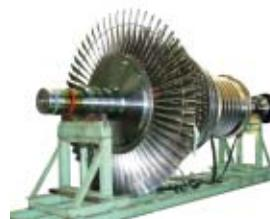
Multistage Steam Turbine Rotor Assembly
