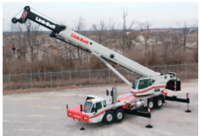
90t Hydraulic Truck Crane
