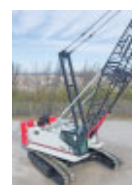
Lattice Crawler Crane
